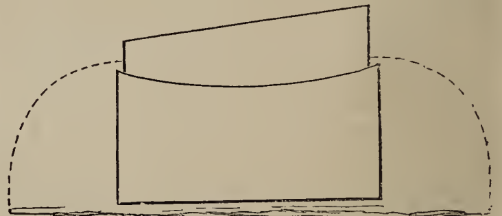
Fig. 1 is a dungbed made in the usual way, with or without faggots, &c., to keep it open, with a frame set upon the top of it. The dotted lines represent the linings to be added when necessary.
